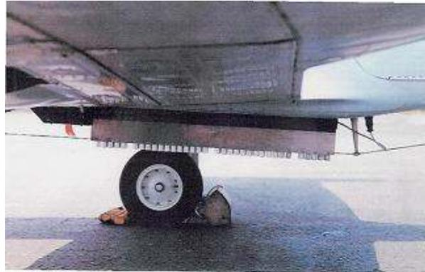
Figure 3 Belly-Mounted Ejectable Flare Rack
