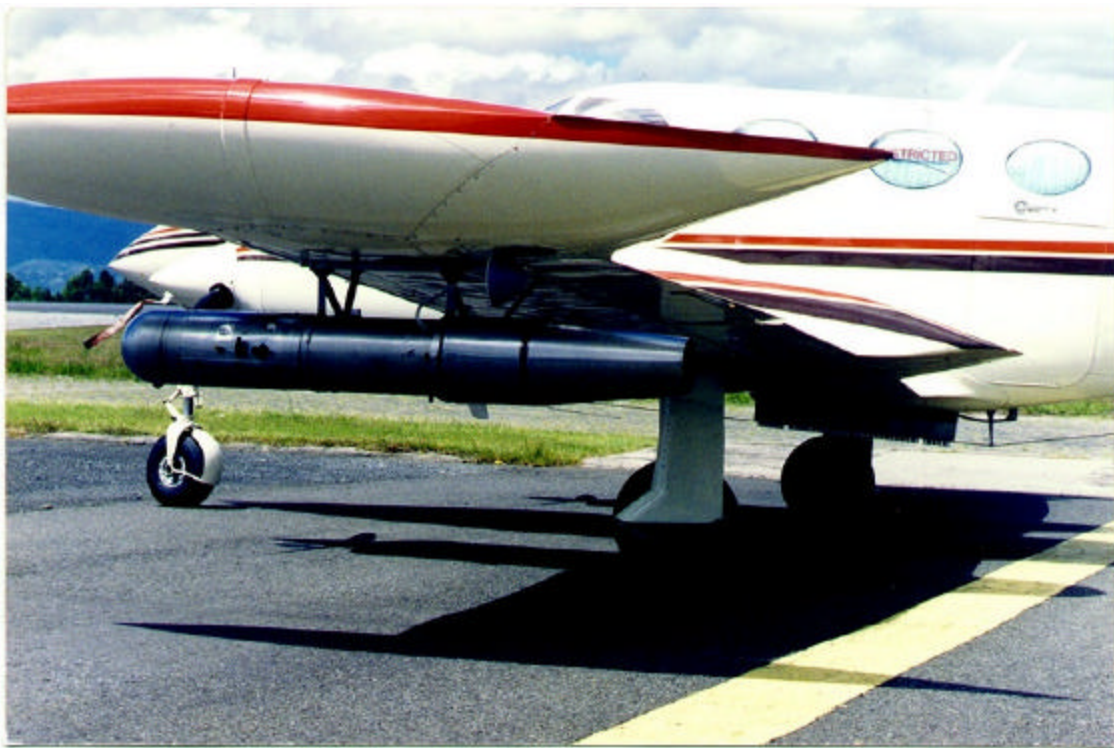
Figure 2 Acetone-Silver Iodide Generator and Droppable Silver Iodide Flare Rack
